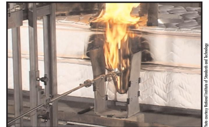
A dual propane burner is used in the CPSC test rig to simulate how burning bedclothes (heat flux and duration) may affect a mattress and box spring or a mattress alone.
