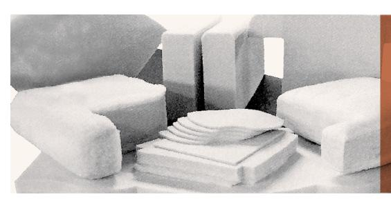
One of the advantages of polyurethane foam is that it can be easily cut, shaped, or combined with other materials to produce cushioning. Foam fabrication can be anything from simple cutting of foam to precise forming and shaping of different components
