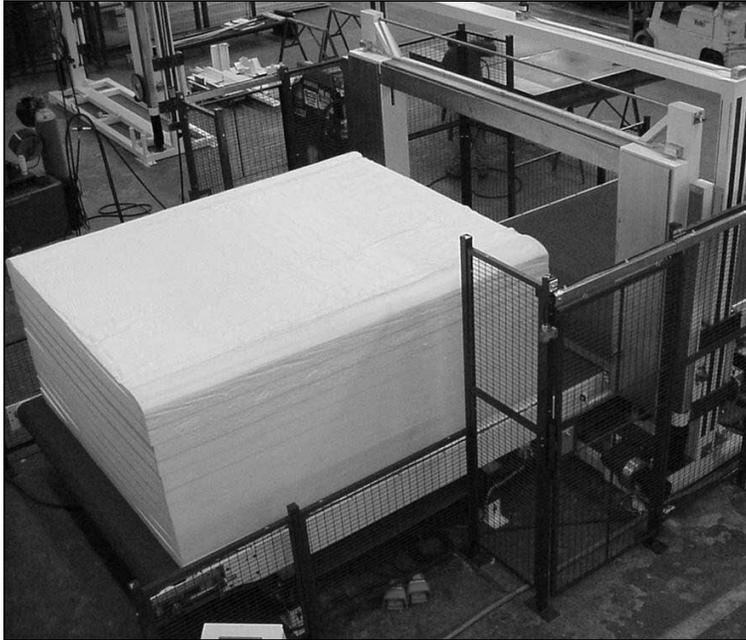
CAD-CNC vertical saws are able to cut buns or sheets and a variety of materials such as FPF, bonded foam and fiber.
