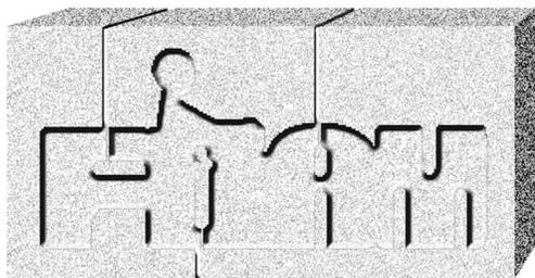
Hot wire cutters can be used to produce intricate shapes. Not all types of FPF lend themselves to hot wire cutting.
