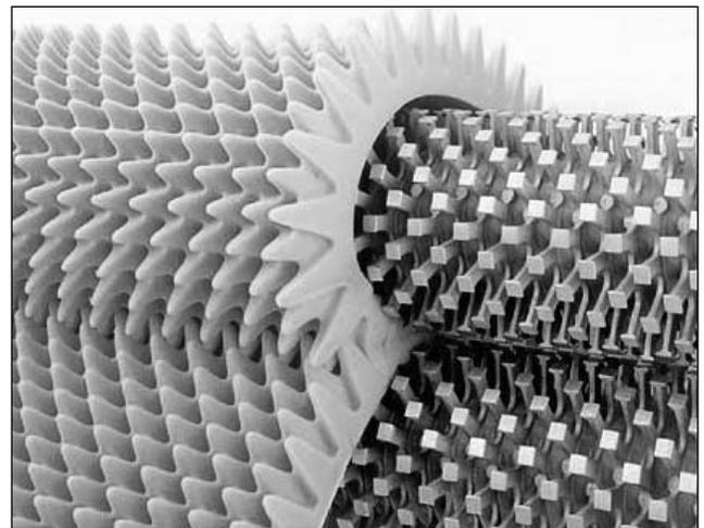
Convoluters use cutting dies to efficiently produce profile shapes from sheets of foam.
