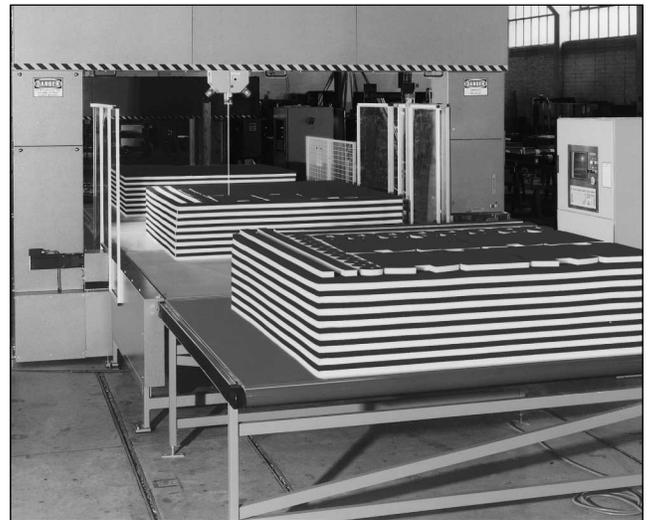
Horizontal slitters allow fabricators to reduce large FPF blocks to sheets.
