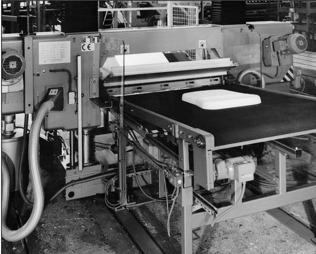
Compression cutting is an efficient alternative to foam molding to produce smooth, contoured shapes.
