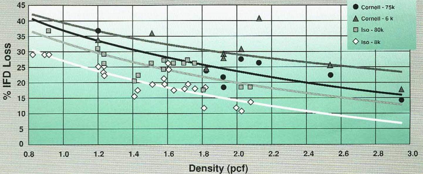
**Firmness change from ASTM dynamic fatigue by roller shear compared to octagonal roller testing**
