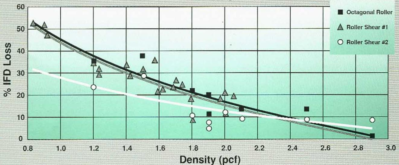
Correlation has been found between test results obtained from small-scale laboratory foam producer testing and full-scale tests used by mattress manufacturers. Small scale tests are routinely performed by foam producers on production samples.
