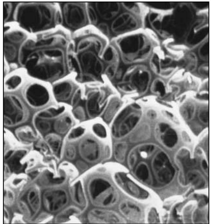
**Flexible foam is a network of tiny interlocking support cells. Each cell is made up of struts and windows. Elastic plastic formed into this unique cellular structure allows the system to compress and recover in response to applied loading and unloading conditions.**
