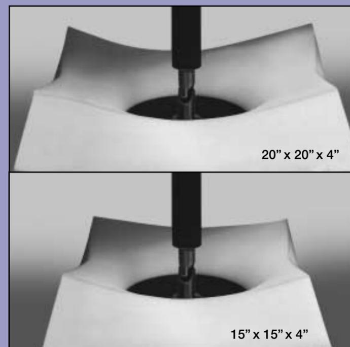
**Sample size can create different "edge effects" in IFD measurement. JIPFC recommends a minimum sample size of 20" x 20" x (purchased thickness) to more closely simulate the natural "edge effect" that occurs in actual cushion use.**
