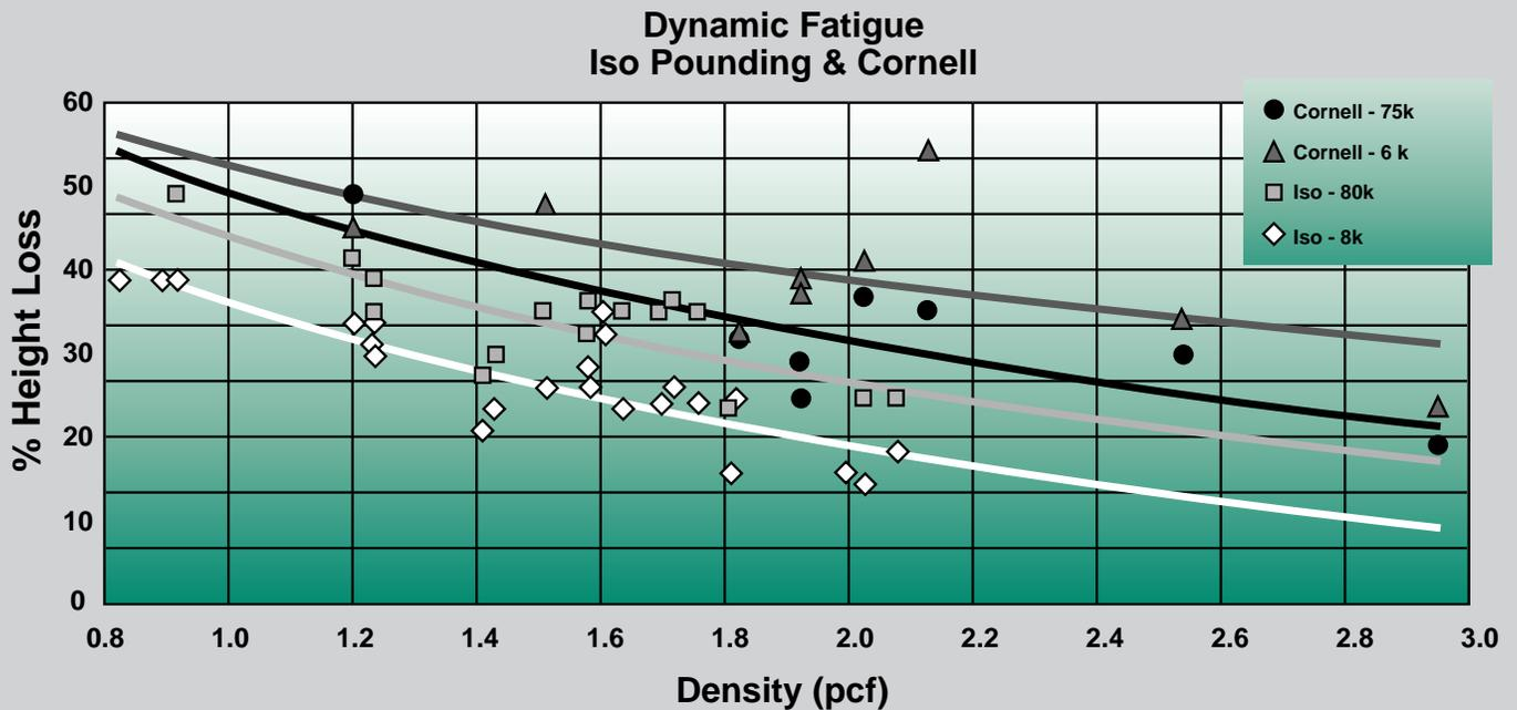
Firmness change from ASTM dynamic fatigue by roller shear compared to octagonal roller testing
