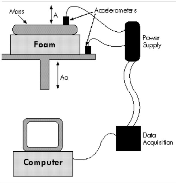
IFD testing uses accelerometers to gather vibrational wave data from the source as well as through different foams to document transmissivity rates over real time.
